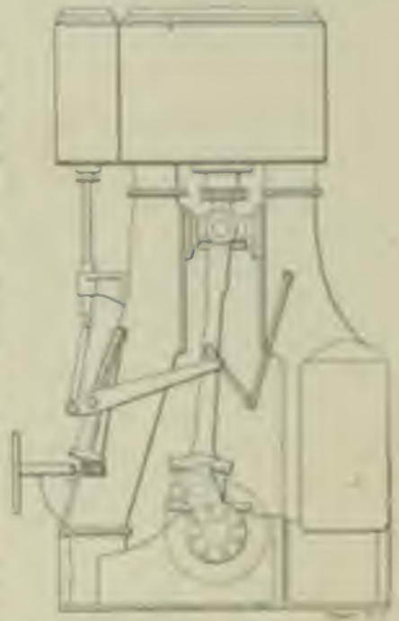
FIG. 19 JOY GEAR APPLIED TO A MARINE ENGINE
